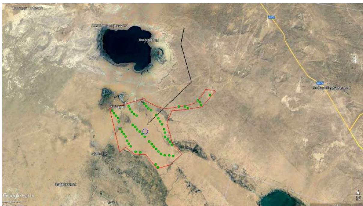
Figure 1. Study area. Red polygon – border of Gijduvan project site, green markers – planned turbine locations, blue circle – substation, black line – OTHL.
