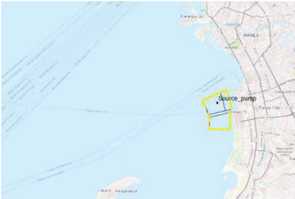
Figure 3-1: Source pump location, inside the Pasay360 Island A+B; sand bunds shown as yellow lines
