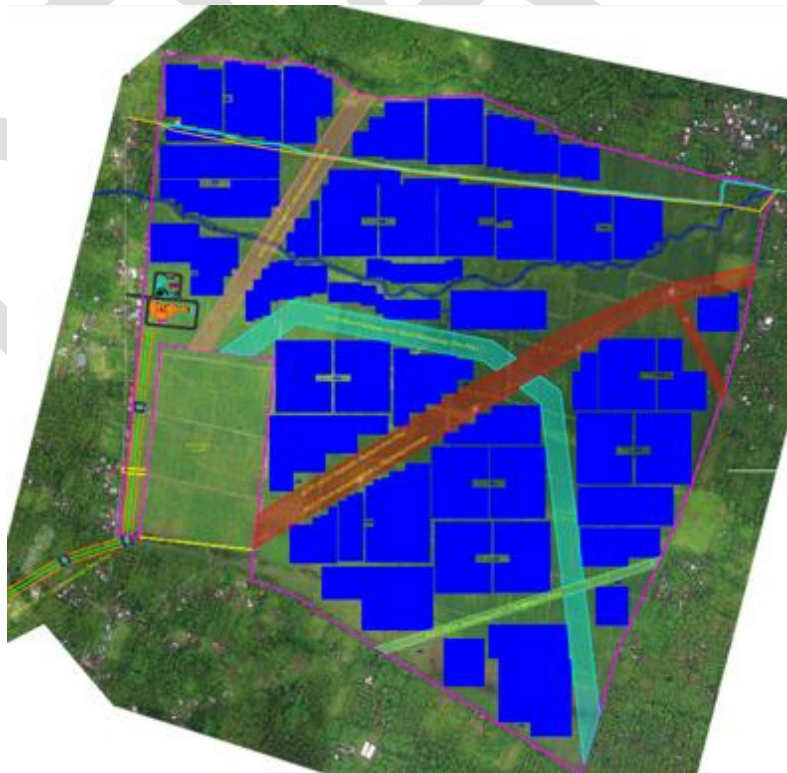
Figure 3-3 Banyuwangi PV Preliminary Plant Layout
