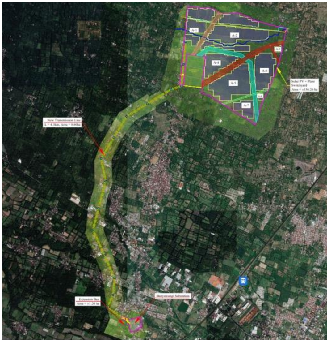
Figure 4-2 Topography survey area Banyuwangi Ground-mounted Solar PV
