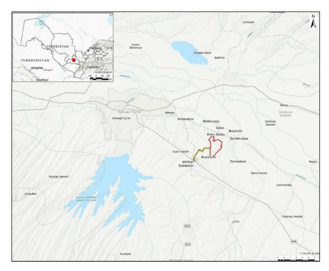
This document covers the development of a 220 MW solar PV project (Project Site) and consists of a Solar PV Site, covering an area of 438 ha, and a 4.5 km Overhead Line from an on-site substation to the existing Ishtihan substation.
