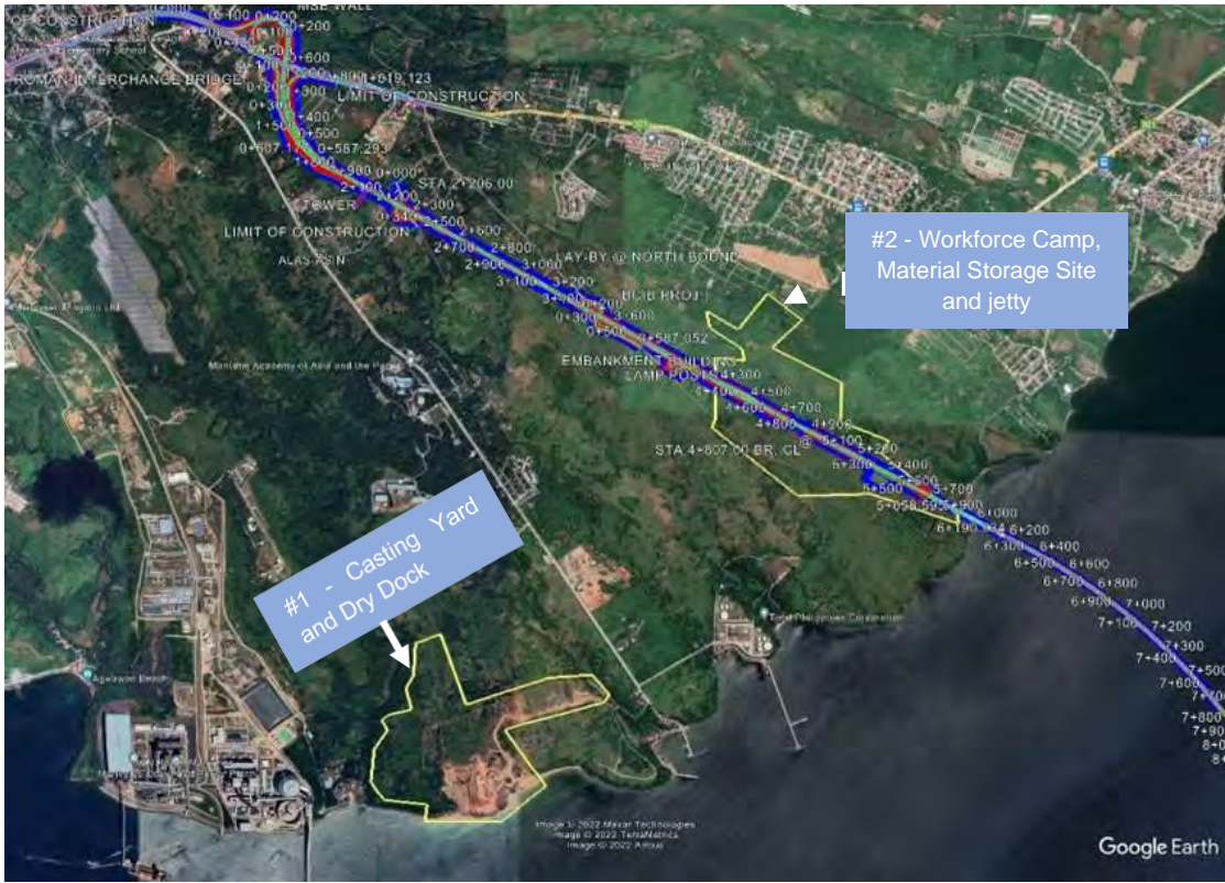
Exhibit 3-21 Bataan Staging Areas and Material Delivery Routes
