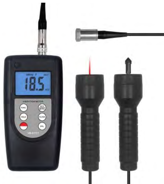
Figure VI.11: Digital Vibration Meter in accordance with ISO 2954
