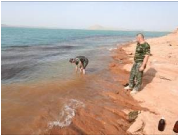
Figure 56: Sampling of Surface Water from The Uchkizil Reservoir at Observation Station SW-01
