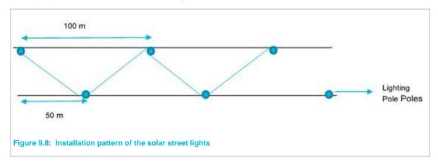
This figure shows the installation pattern of the streetlight alongside the road at the project boundary and as well as in the internal road network, in the facility. The blue dot represents the streetlight, in the picture. In case of single facility like pump house, ETP and other open facilities, where a focused illumination is necessary, one or two poles of light would be separately installed in the close proximity of the unit.
