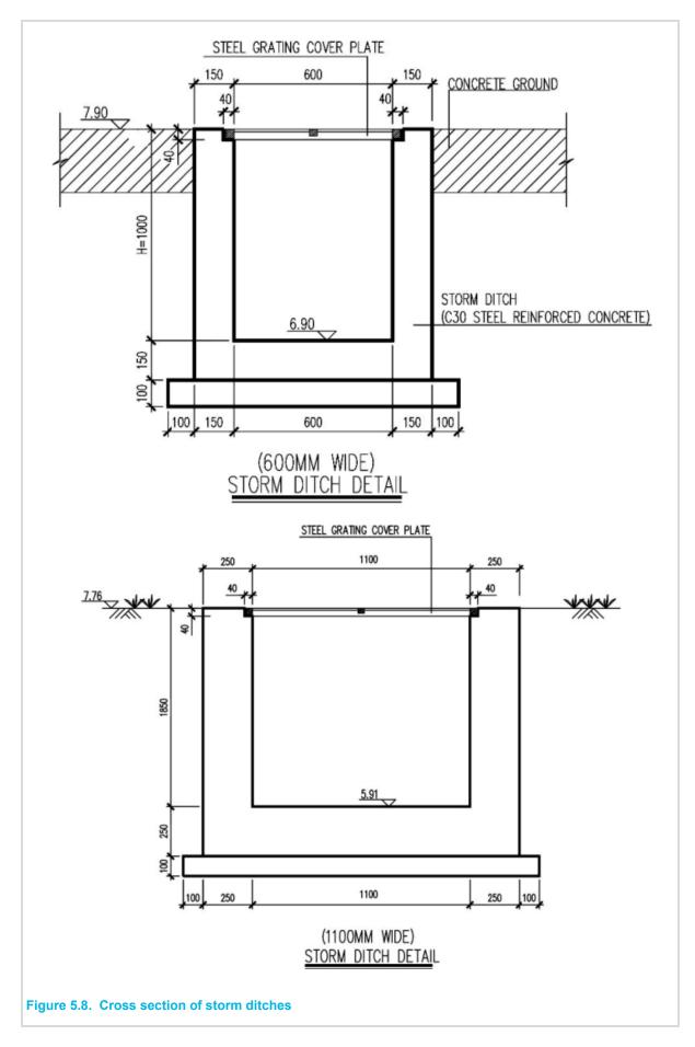
The yard area of the proposed project would be provided with a 2% slope and the steeper shoulder slope of 2.5 %, to drain away water through the drainage channels. A minimum of 1% slope would be provided for the flow of
