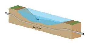
floods. Factors that control scour are the river flow, the characteristics of the riverbed and riverbank sediments, and the capacity of the river to transport sediments. Construction or other changes upstream and downstream of a pipeline crossing can influence river flow and channel morphology.
