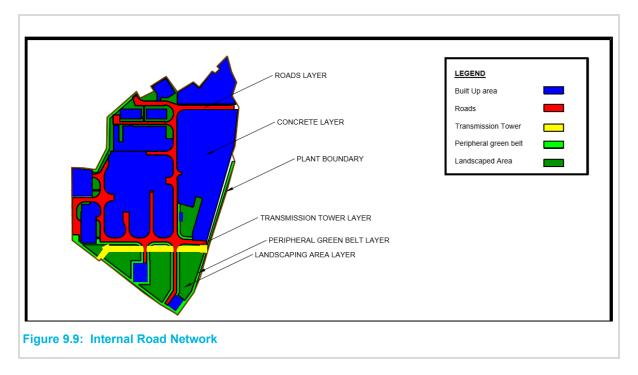
The total area of internal roads is approx. 11,221 sq. m with length of the road being approx. 1675 m. The width of the road varies along the entire stretch as shown in Figure 2. From Figure 2, it is understood that there are 9 intersections on the internal road network, where the width of the road is more. Therefore, it is assumed that at 9 intersections and peripheral boundary, total 30 streetlights would be installed
