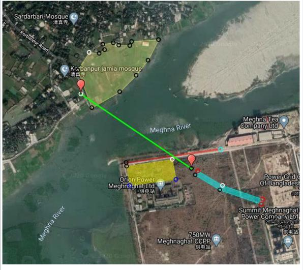
Figure 3.27: Option 2-General alignment of the Pipeline HDD
