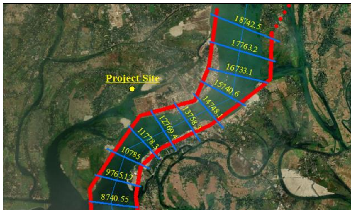
Figure 7.15.Channel in front of project site as well as its cross sections
