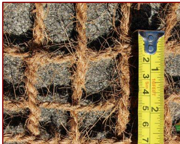
Coir geo-textiles specifications: Grade I- 400g/m 2
