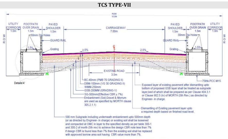
TYPICAL CROSS SECTION FOR TWO LANE WITH PAVED SHOULDER, AND FOOTPATH OVER DRAIN BOTH SIDES(BUILT-UP AREA)
