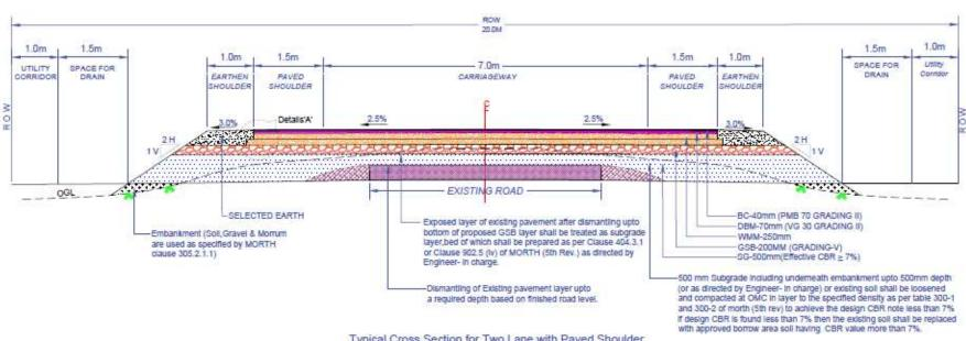
Typical Cross Section for Two Lane with Paved Shoulder and Earthen Shoulder.
