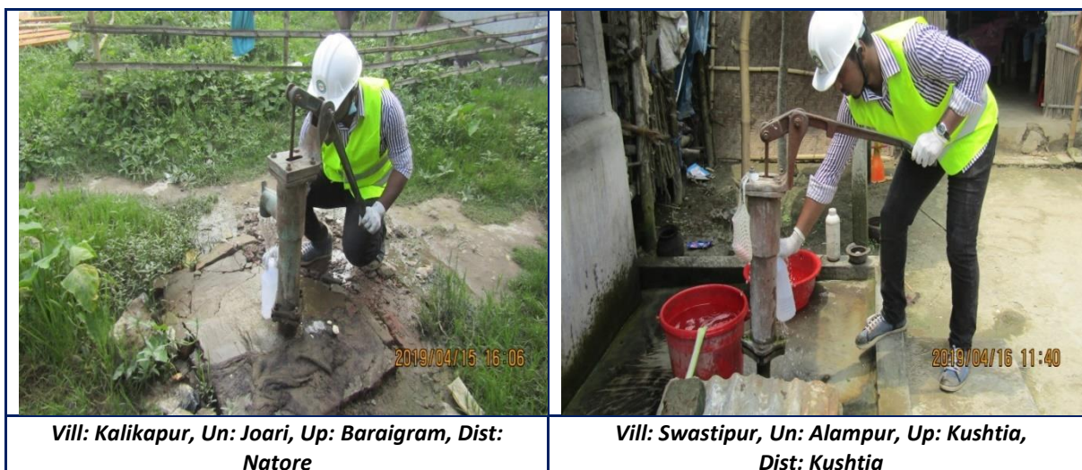
Figure IV-22: Sampling of Groundwater in the Project Area
