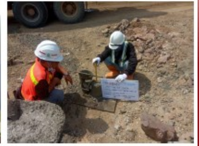
Checklist & Slump Test Slab Tank 2 East GWT
