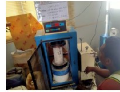
7 days Compressive Strength Test of f'c 25 Mpa Integral Waterproofing Column Tank 1 West GWT
