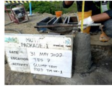
Checklist & Slump Test Rigid Pavement Roundabout Tes 7
