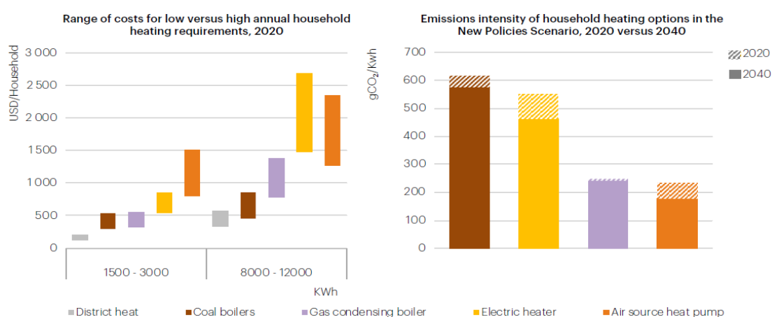
Figure A3.1: Heating Costs and Emissions Intensity of Different Technologies
