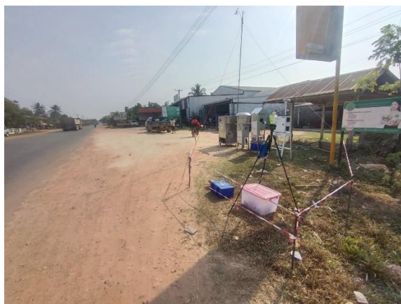
Plate 5-8: Vibration monitoring at AQ02
